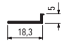
650 101 Edge protection 567 257.17 Push-in gasket Material: Plastic Surface finish: Silver PU: 100 running metres
